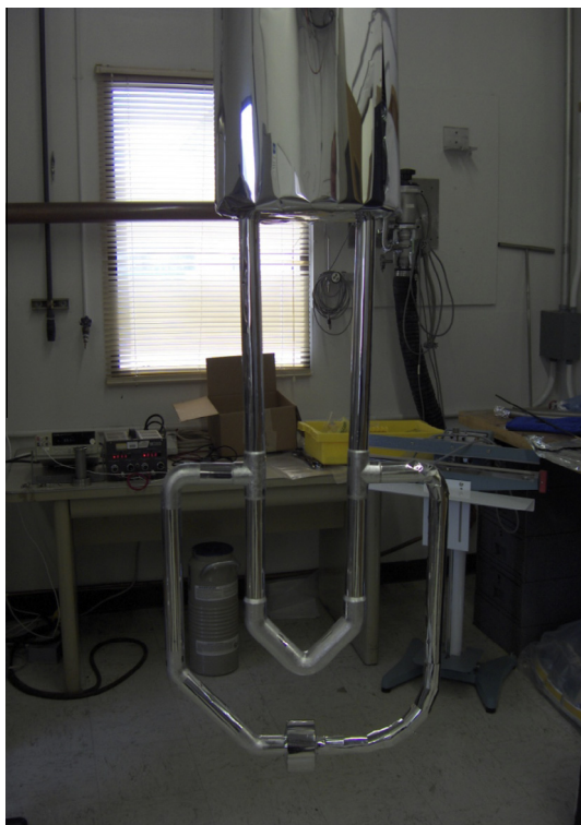
Fig. 8. WMLI installed on complex geometry tubing set – containing 45°, 90° bends, T's, flanges and sweeping corners – for LN 2 boil-off calorimetry.
