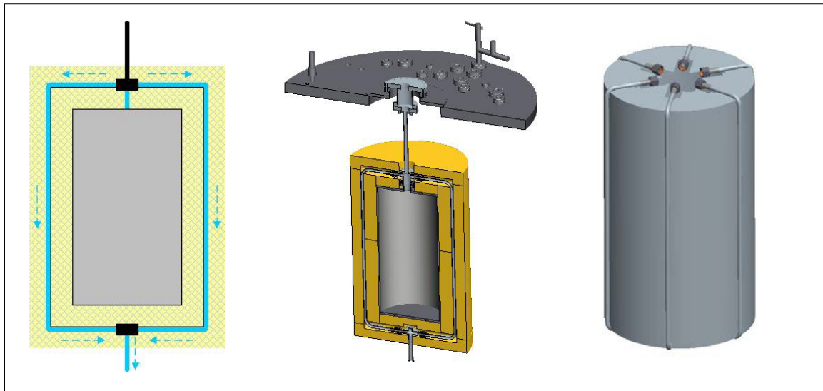
Figure 1: Boil-off path diagram, test article CAD images
