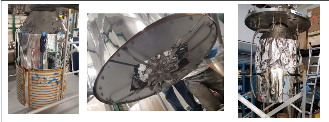
Figure 11: (left) 400L tank skirt with serpentine cooling flow; (middle) lower manifolding for cooling flow channels; (right) fully-assembled 400L test article with IMLI
