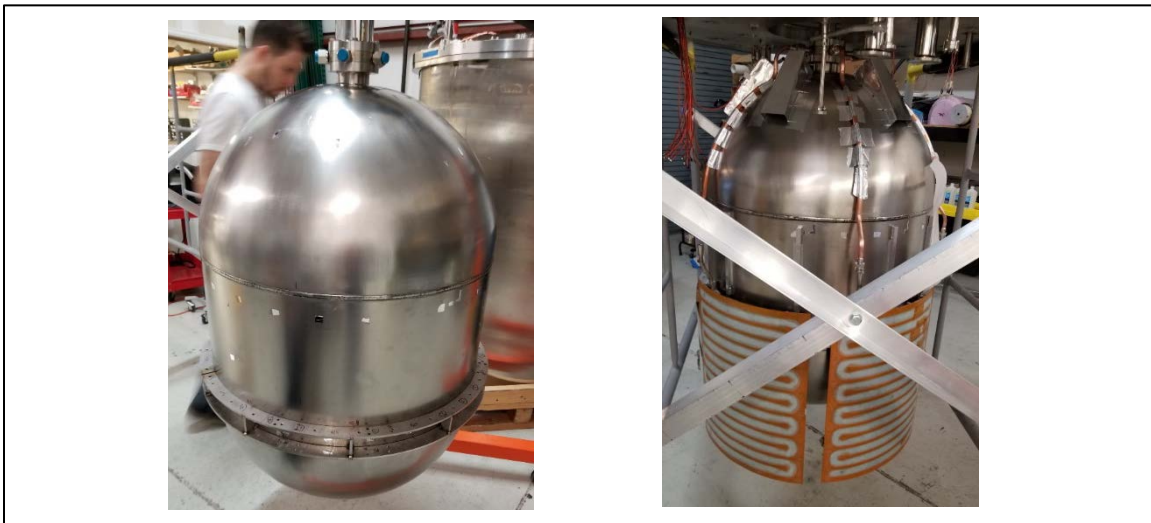
Figure 10: (left) 400L tank with girth ring; (right) test article assembled prior to IMLI install
