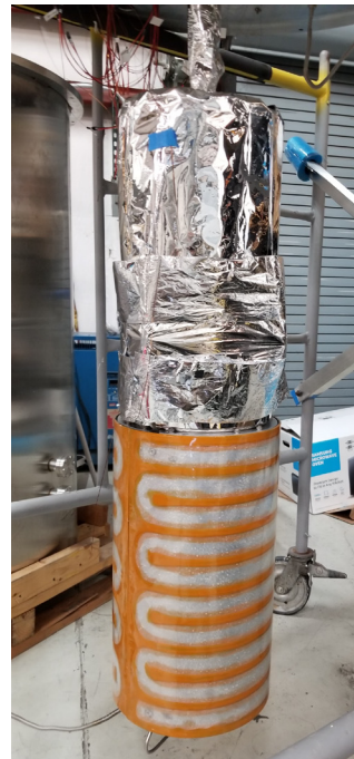
Fig 7. Panels installed on Phase II 20L tank/skirt prototype.
