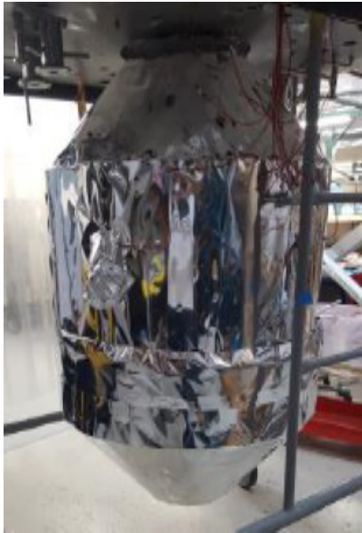
Fig 8. 400L VCS tank baseline test configuration
