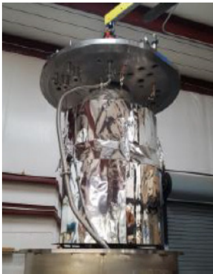
Fig 9. VCS 400L test fixture in 100% cooled & insulated configuration; skirt panels installed with heater plates and 100% surface cooling
