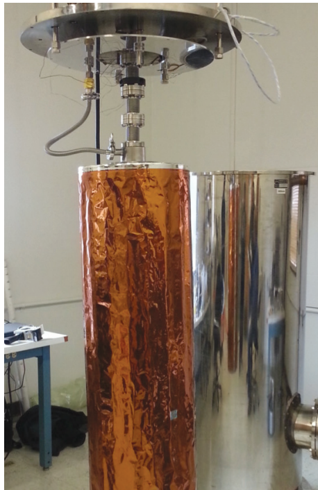
Launch Vehicle-Load Responsive MLI prototype ready for thermal testing (polymer laminate vacuum shell visible). Image: Quest Thermal Group
