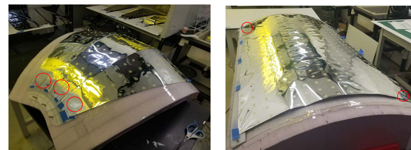
Approximate metallized spacer location (red circles) for cryogenic tank dome (left) and barrel section (right)
