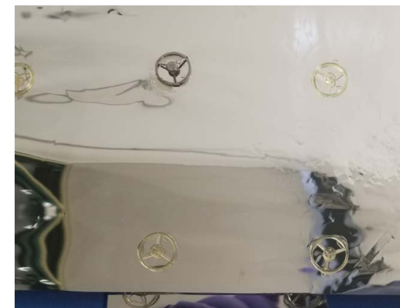
VDA metallized spacers bonded to radiant barriers
