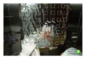
Figure 1. In this Prototype Assembly, a discrete matrix comprising a square array of square frames is placed on a metallized polymer film. In constructing a multilayer insulation blanket, arrays like this one would be placed between all the metallized polymer film layers.
