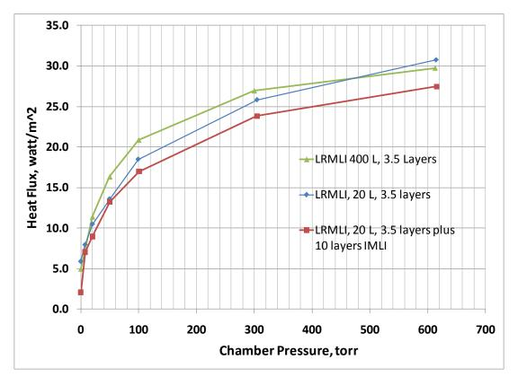
Figure 3. LRMLI heat leak from 295°K to 77°K as a function of external atmospheric pressure.
