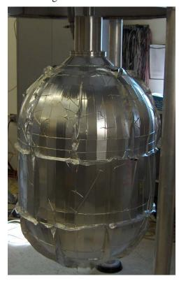
inches in diameter and 24 inches long. The tank was tested with the LRMLI and then with 10 layers of integrated MLI applied over the LRMLI.
