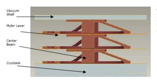
with lower conducted heat leak. Figure 1 shows a cross section view of a three layer version of LRMLI. The two stage feature of the posts can be seen.
