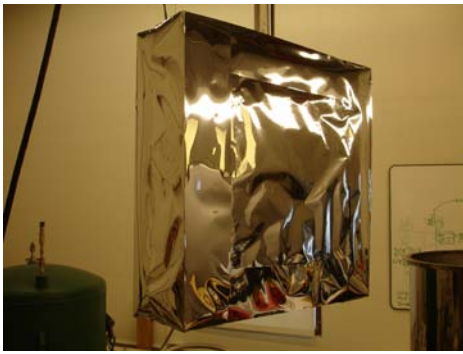
FIGURE 3. Calorimeter test tank insulated with IMLI.
