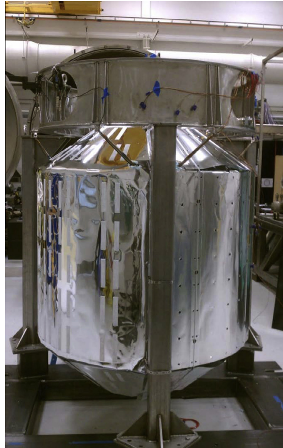
Fig. 6. LBMLI installed on VATA tank at NASA Marshall; left half is LBMLI, right half has BAC shield installed.
